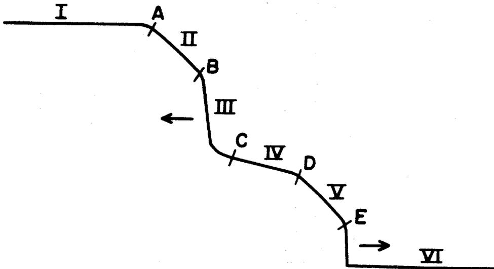
Fig. 2. Schematic temperature distribution. I, isothermal sphere; III, cooling wave; VI, undisturbed air; E, shock front. II, IV, and V are expanding adiabatically.
