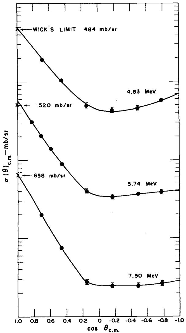
Fig. 4. The differential neutron elastic scattering cross sections for  ${}^6\text{Li}$  in the center-of-mass system. The curves are visual fits to the data. Note the discontinuities in the vertical scale.
