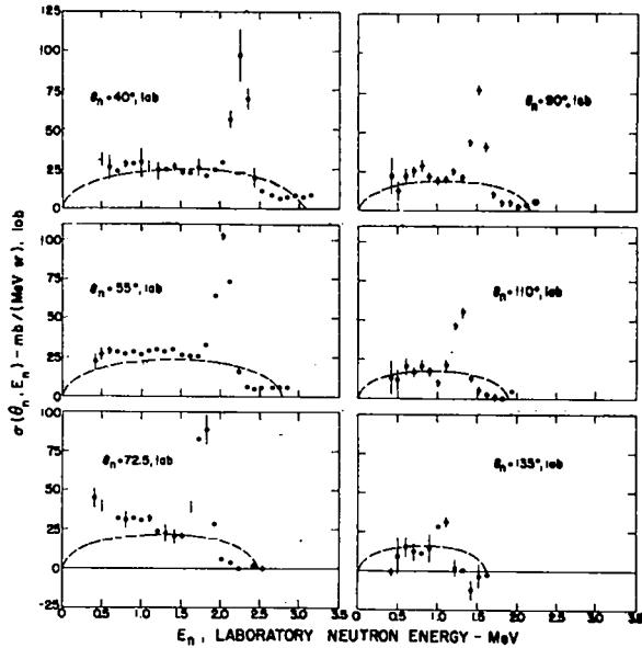
Fig. 2. Energy spectra of neutrons inelastically scattered from  $^{6}\text{Li}$  at an incident neutron energy of 4.83 MeV. The dashed curves represent the distributions obtained from a three-body phase space calculation normalized to the total  $^{6}\text{Li}(n, dn)^{4}\text{He}$  cross section obtained in the present experiment.
