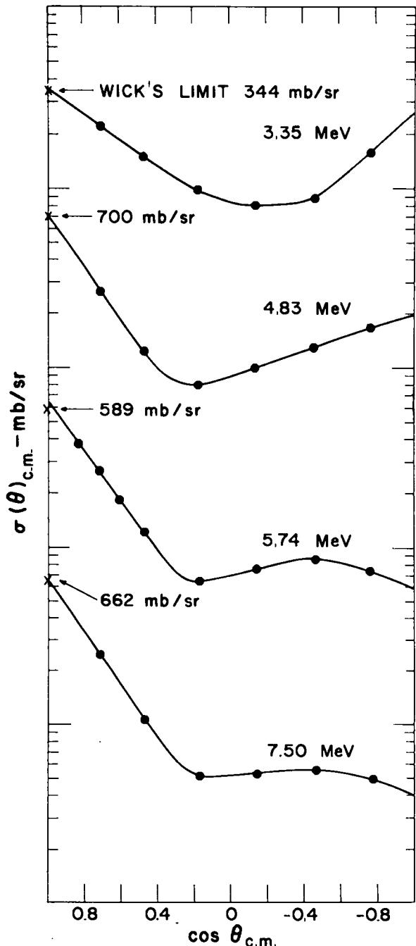
Fig. 8. The differential neutron elastic scattering cross sections for  ${}^7\text{Li}$  in the center-of-mass system. The 5.74- and 7.5-MeV data include the scattering to the first excited state at 0.478 MeV.
