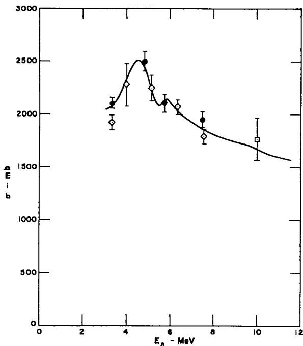
Fig. 9. Total cross sections for  ${}^7\text{Li}$  versus incident neutron energy.
