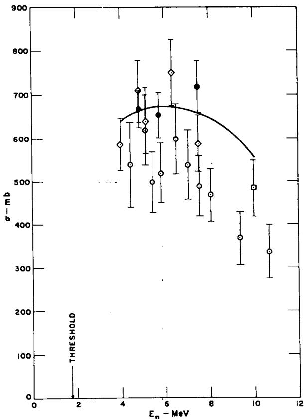
Fig. 7. The  ${}^6\text{Li}(n, \text{dn}){}^4\text{He}$  cross section as a function of incident neutron energy.
