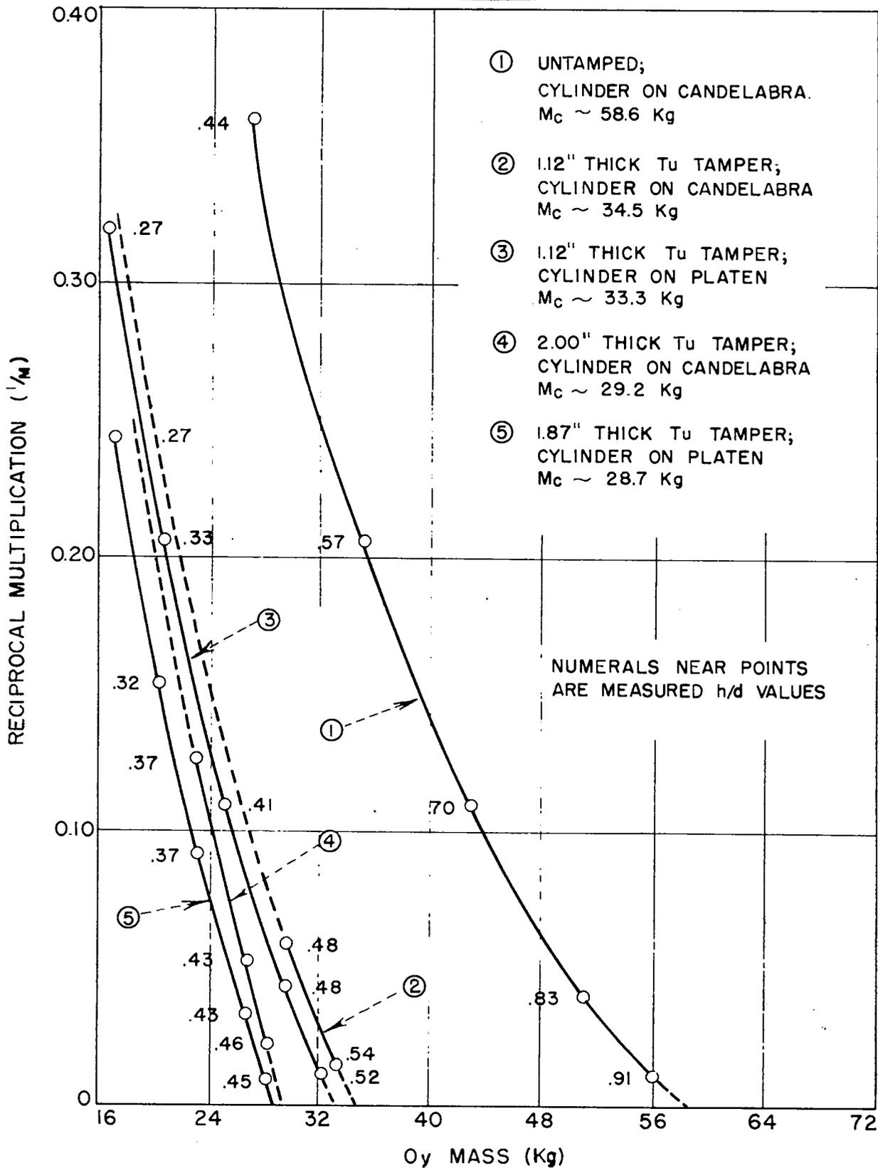
FIG. 10 RECIPROCAL MULTIPLICATION MEASUREMENTS
