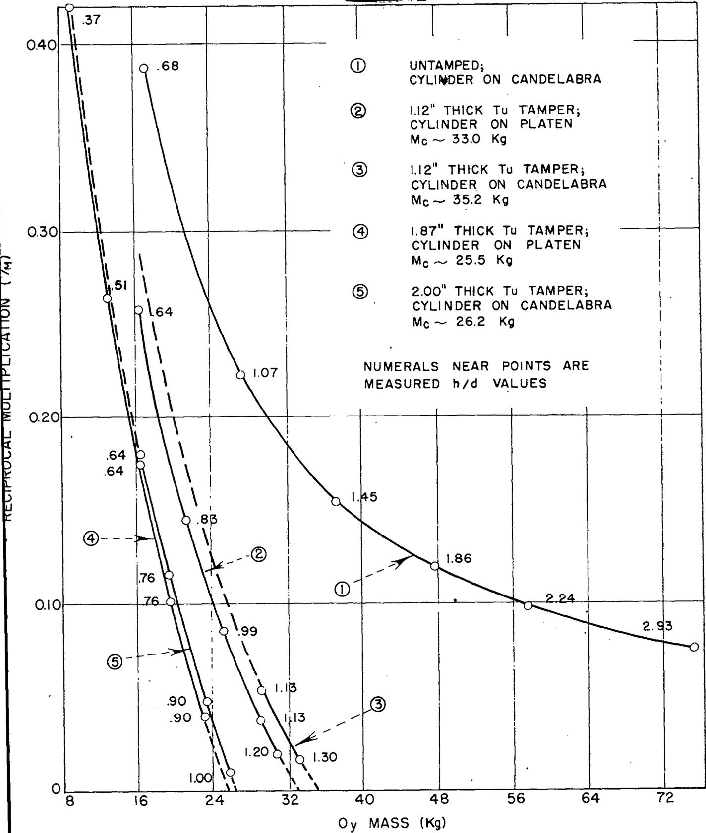
FIG. 8 RECIPROCAL MULTIPLICATION MEASUREMENTS
