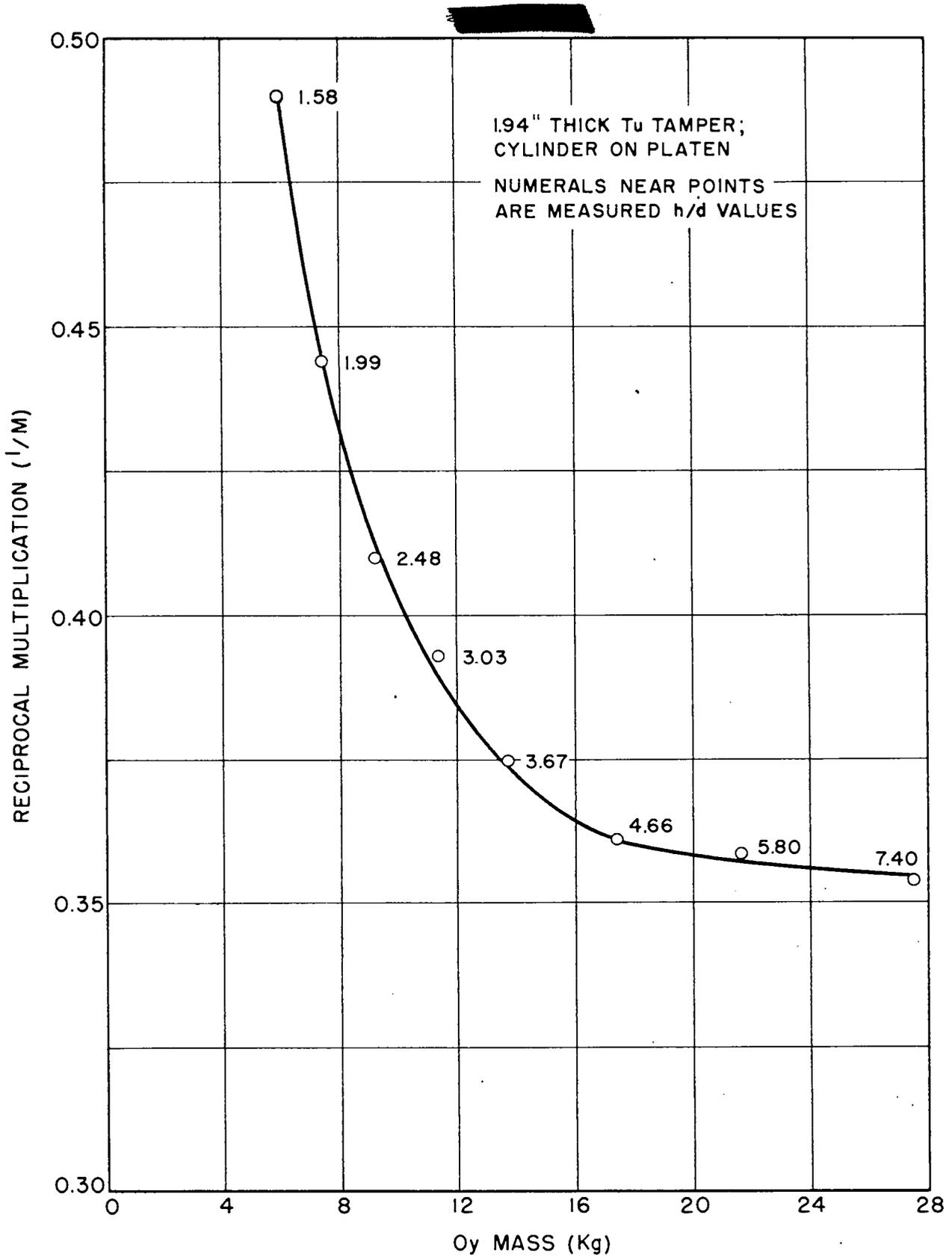
FIG. 5 RECIPROCAL MULTIPLICATION MEASUREMENTS ON 2.50" DIAMETER Oy CYLINDER
