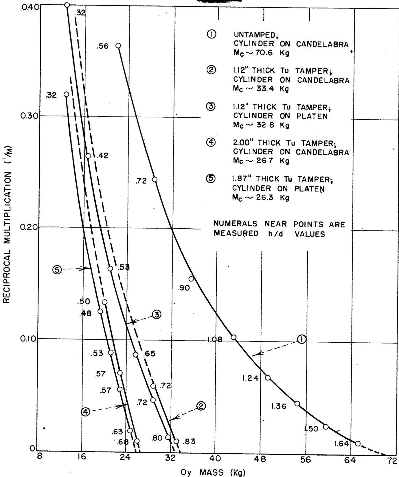
FIG. 9 RECIPROCAL MULTIPLICATION MEASUREMENTS ON 5.50" DIAMETER Oy CYLINDERS
