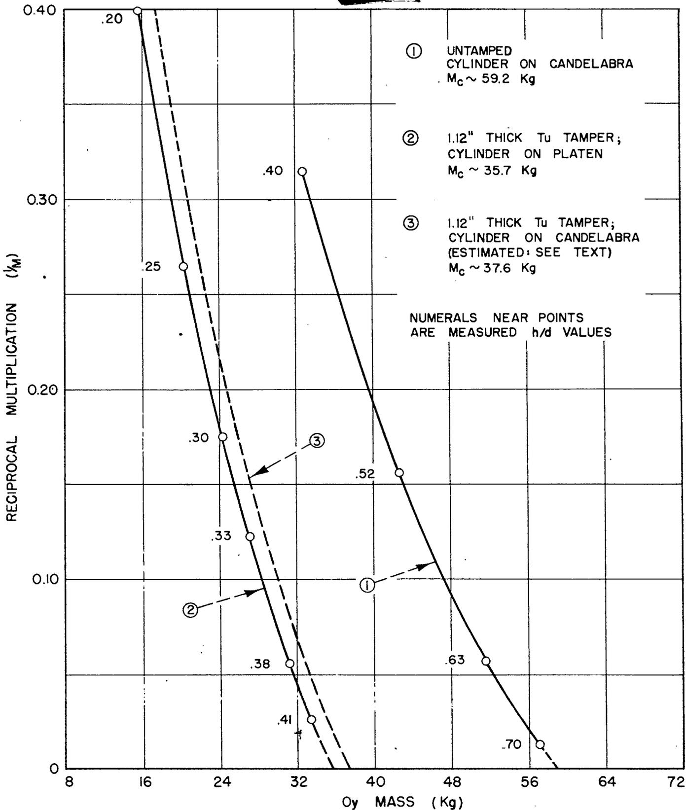
FIG. II RECIPROCAL MULTIPLICATION MEASUREMENTS ON 7.00" DIAMETER Oy CYLINDERS
