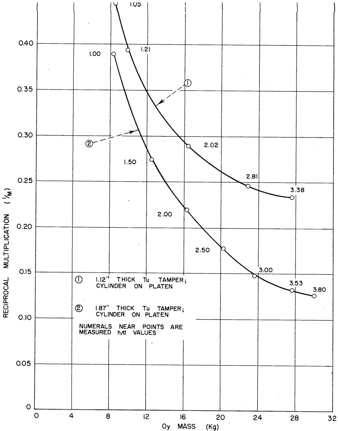
FIG. 6 RECIPROCAL MULTIPLICATION MEASUREMENTS ON 3.25" DIAMETER Oy CYLINDERS
