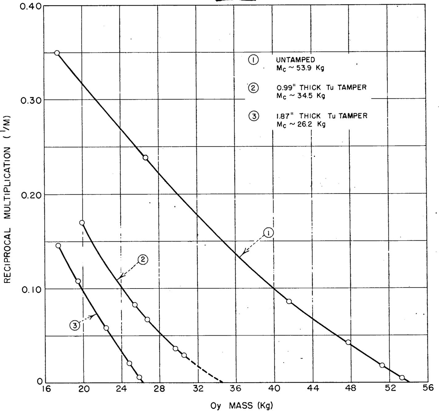
FIG. 14 RECIPROCAL MULTIPLICATION MEASUREMENTS ON Oy PSEUDOSPHERES
