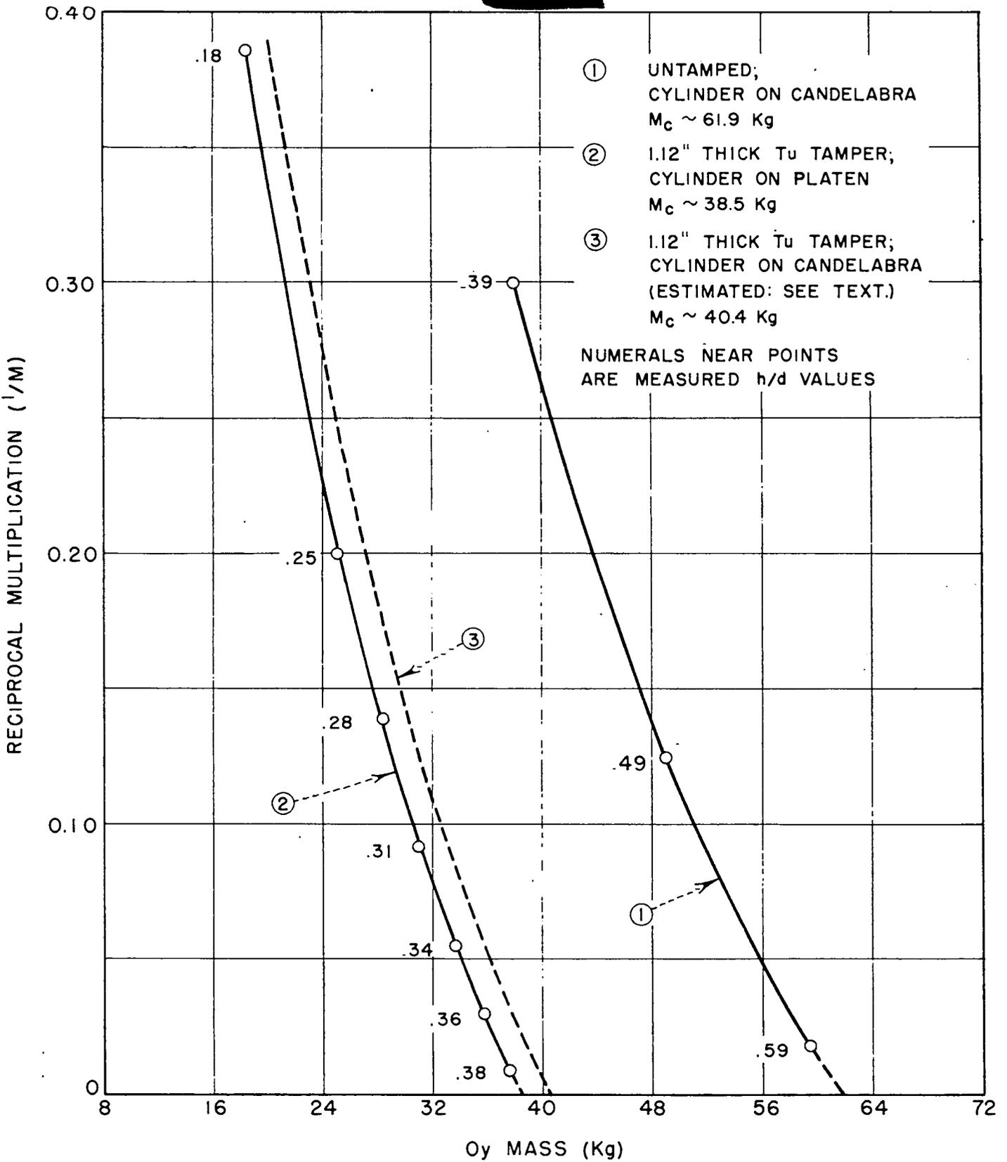
FIG. 12 RECIPROCAL MULTIPLICATION MEASUREMENTS ON 7.50" DIAMETER Oy CYLINDERS
