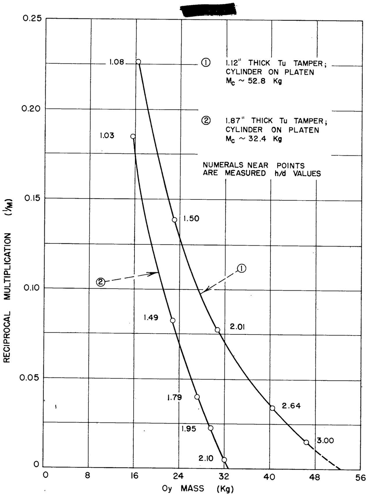
FIG. 7 RECIPROCAL MULTIPLICATION MEASUREMENTS ON 3.98" DIAMETER Oy CYLINDERS
