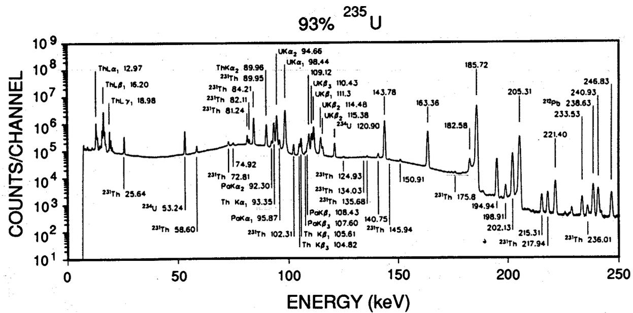
Fig. 1.8 Gamma-ray spectrum of highly enriched uranium showing the intense gamma rays often used for assay of <sup>235</sup>U.
