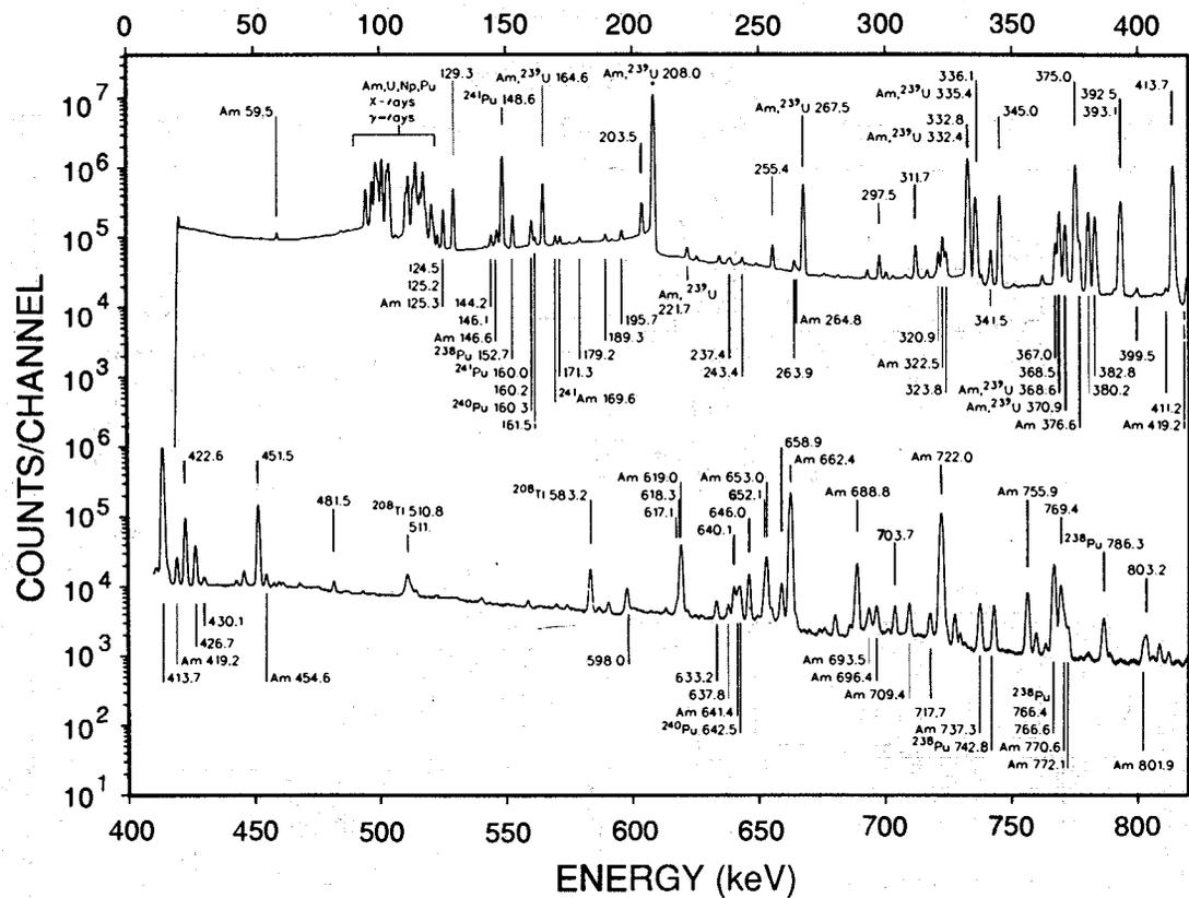
Fig. 1.10 Gamma-ray spectrum of plutonium with 14%  $^{240}\text{Pu}$  and 1.2%  $^{241}\text{Am}$ . Compare this spectrum with that of Figure 1.11, noting the difference in relative intensities. Compare the intensities of the gamma rays at 203.5 keV ( $^{239}\text{Pu}$ ) and 208.0 keV ( $^{237}\text{U}$ , daughter of  $^{241}\text{Pu}$ ).
