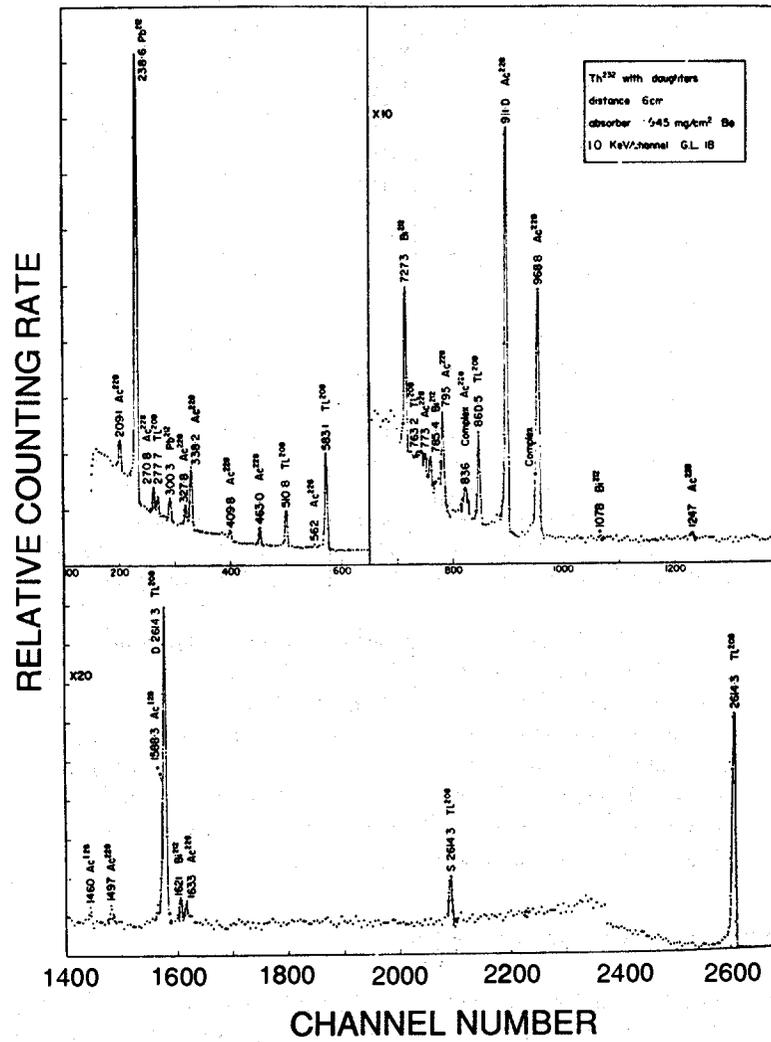
Fig. 1.12 Gamma-ray spectrum of  $^{232}\text{Th}$  and its daughter products. Thorium-232 emits no significant gamma rays of its own. The daughter nuclides grow into equilibrium with the  $^{232}\text{Th}$  parent over a period of approximately 35 yr. [Figure adapted from F. Adams and R. Dams, Applied Gamma-Ray Spectroscopy, 3rd ed. (Pergamon Press, Oxford, 1970).]
