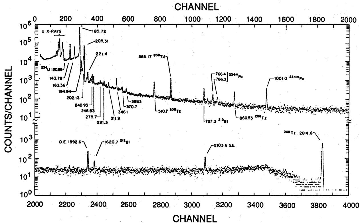
Fig. 1.7 High-resolution gamma-ray spectrum of highly enriched uranium (93%  $^{235}\text{U}$ ). Energies are given in kiloelectron volts. (S.E. and D.E. are the single- and double-escape peaks of the 2614-keV gamma ray.)
