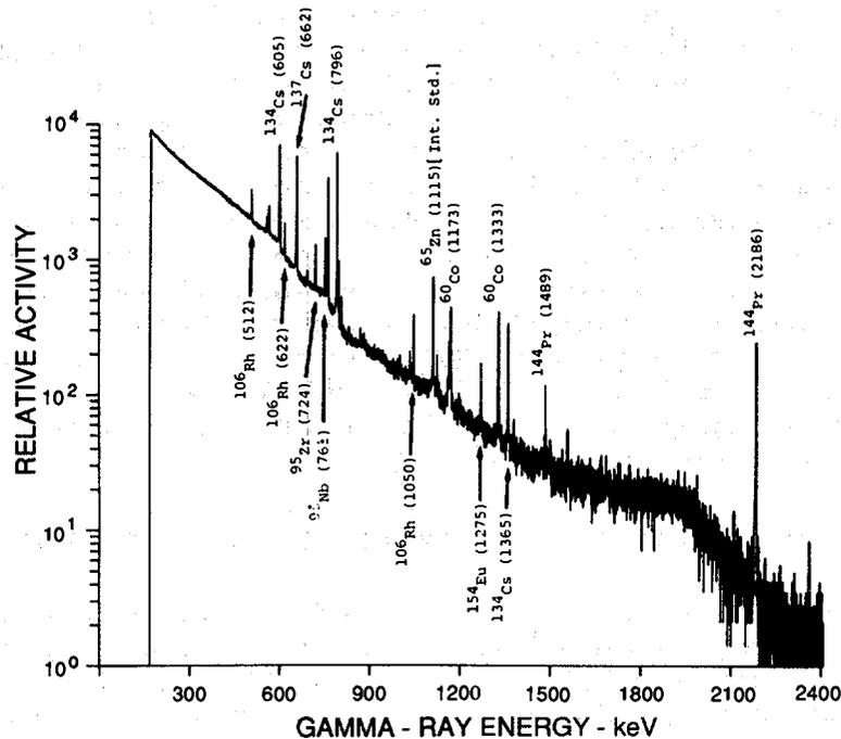
**Fig. 1.14** Gamma-ray spectrum of irradiated pressurized-water-reactor fuel having a burnup of 32 000 MWd/tU (megawatt days per ton of uranium) and a cooling time of 9 months.
