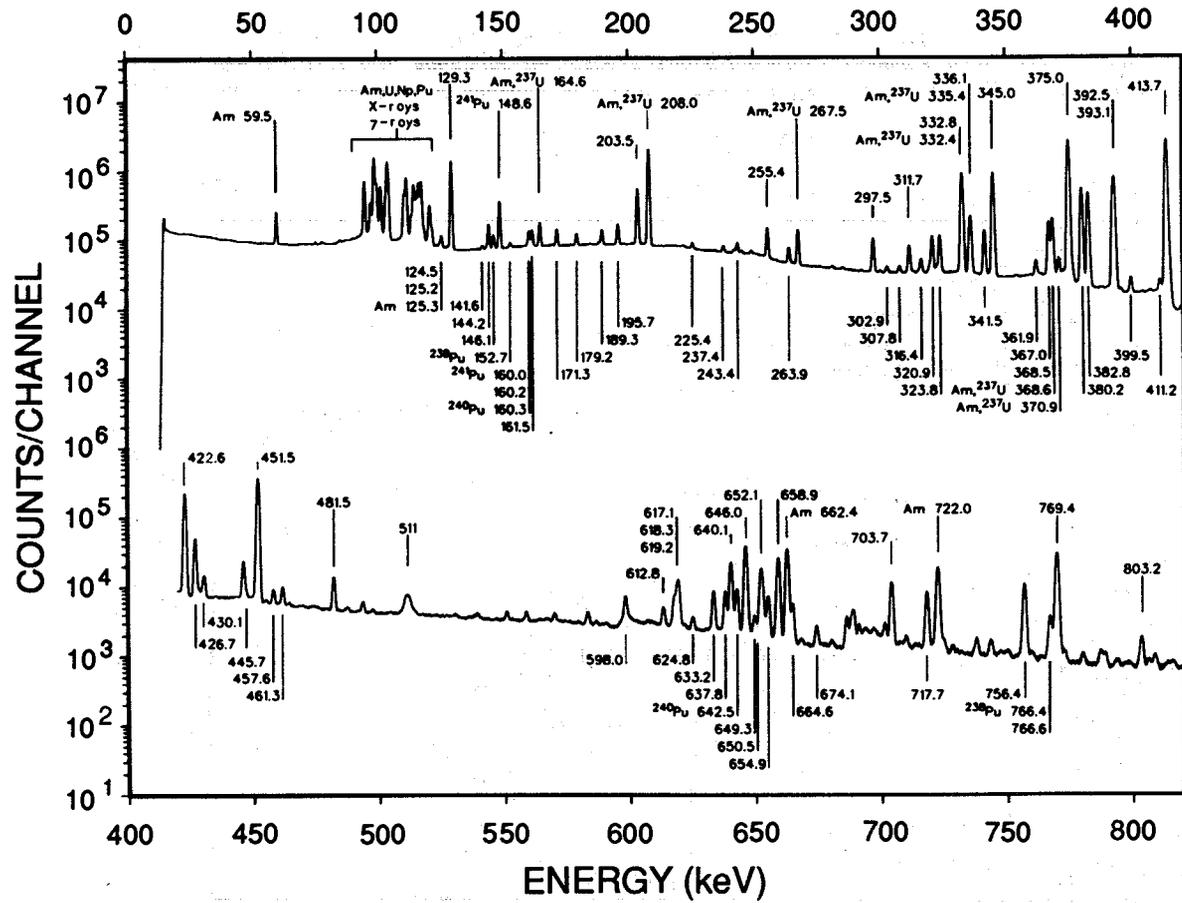
Fig. 1.11 Gamma-ray spectrum of low-burnup plutonium with approximately 6% <sup>240</sup>Pu.
