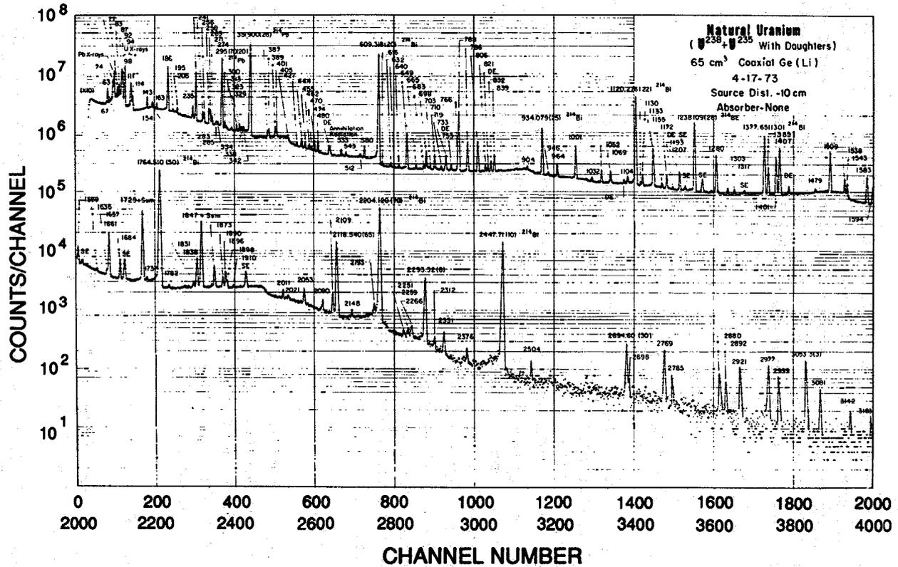
Fig. 1.15 Gamma-ray spectrum of uranium ore. Major radiations are from  $^{214}\text{Pb}$  and  $^{214}\text{Bi}$ . Compare the spectrum of processed uranium fuel in Figure 1.9; most daughter products are removed during processing. Figure adapted from R. L. Heath, "Gamma-Ray Spectrum Catalogue," Aerojet Nuclear Corporation report ANCR-1000-2 (March 1974).
