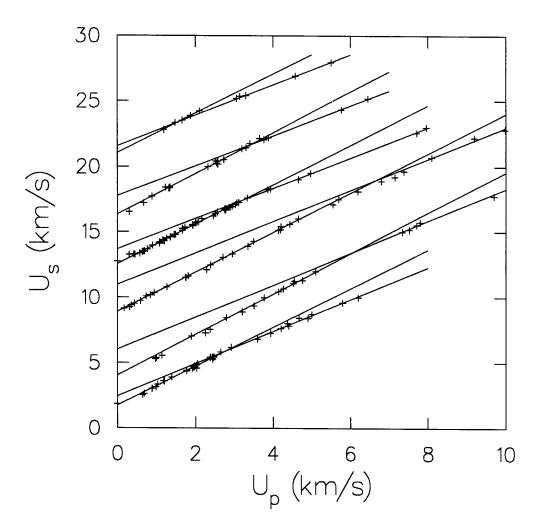
Fig. 4. Bi, Fe, Cu, Sn, Ar, and Xe Hugoniot data from bottom to top. Shifts have been introduced to avoid overlaps.
