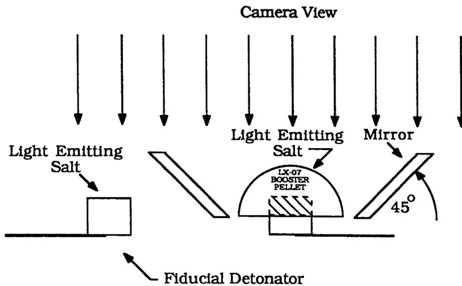
Fig. 3. Schematic of wave-emergence experiment for LX-07 17-mm hemispherical booster pellet.
