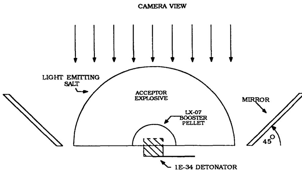
Fig. 1. Schematic of typical Los Alamos onion-skin test.
