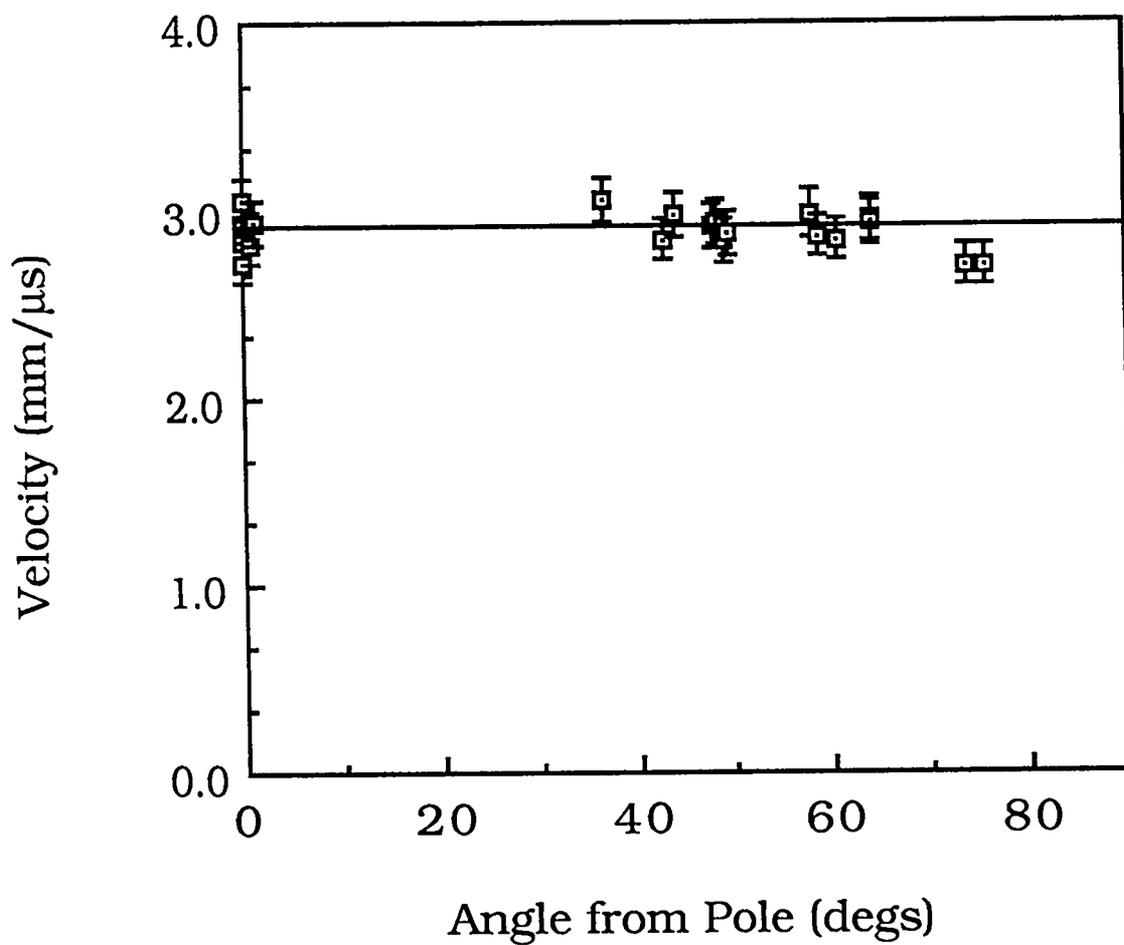
Fig. 15. Interface jump velocities for PMMA window 1 LX-07 pellet interface versus the radial angle from the hemisphere pole. Solid line represents the Chapman-Jouguet detonation model prediction.
