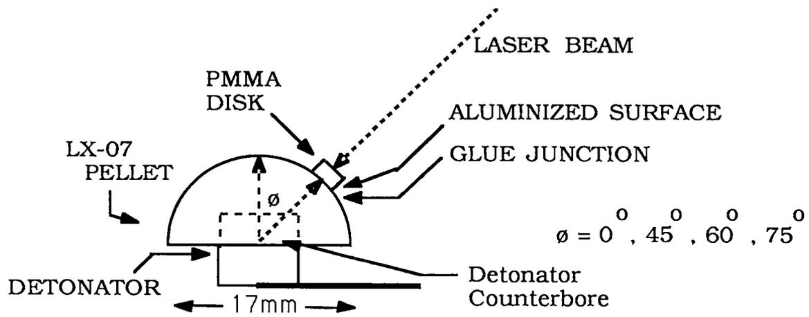
Fig. 5. Schematic of the velocity measurement experiments.
