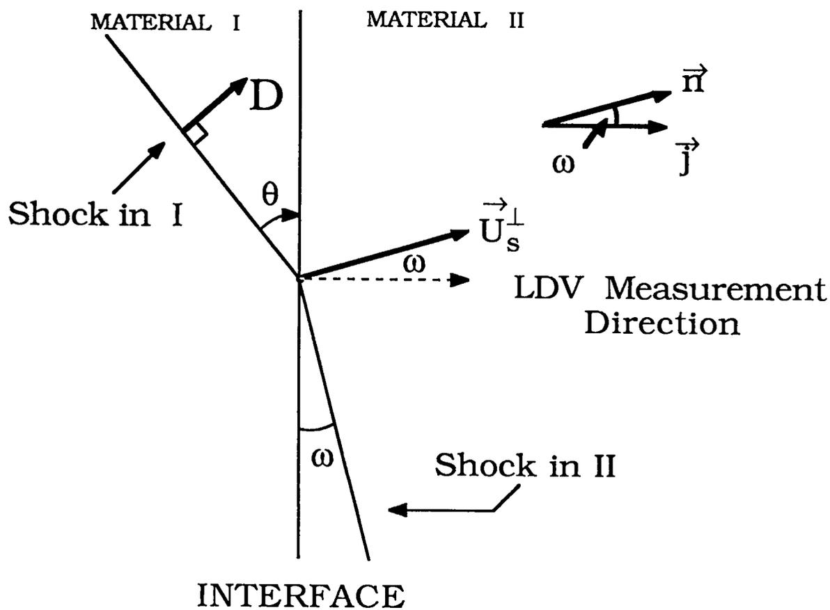
Fig. 16. Idealization of the interaction of a shock wave at the interface between two dissimilar materials.
