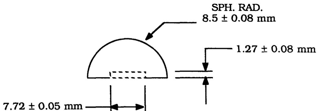
Fig. 2. Design parameters for the LX-07 hemispherical booster pellet.
