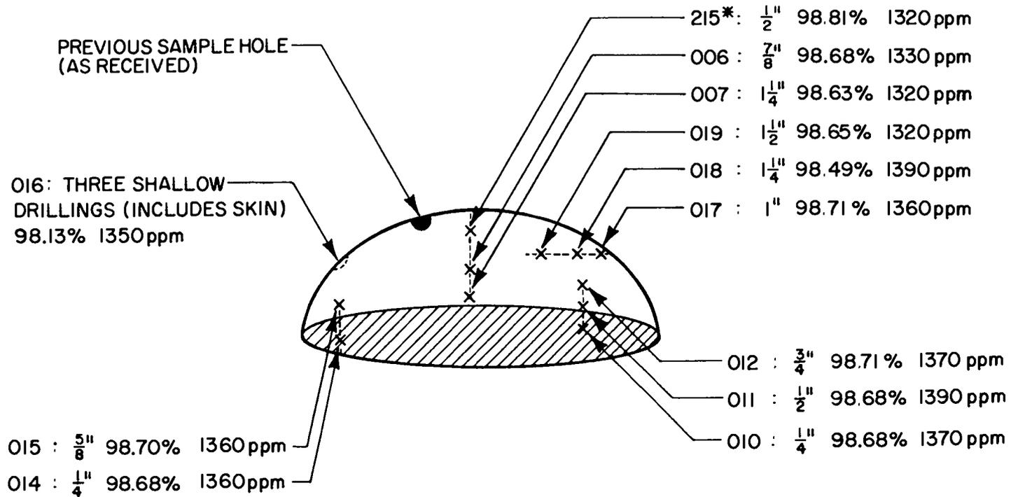
USING A HYDRAULIC CHISEL, THREE PIECES WERE SHEARED OFF THE BUTTON. IT IS NOT POSSIBLE TO PINPOINT THE LOCATION OF THESE SAMPLES. THEY ARE:
