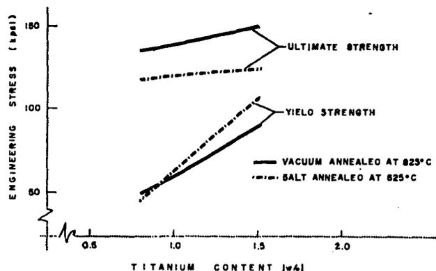
Fig. 1 Mechanical Strength vs Titanium Content For Uranium-Titanium Alloys
