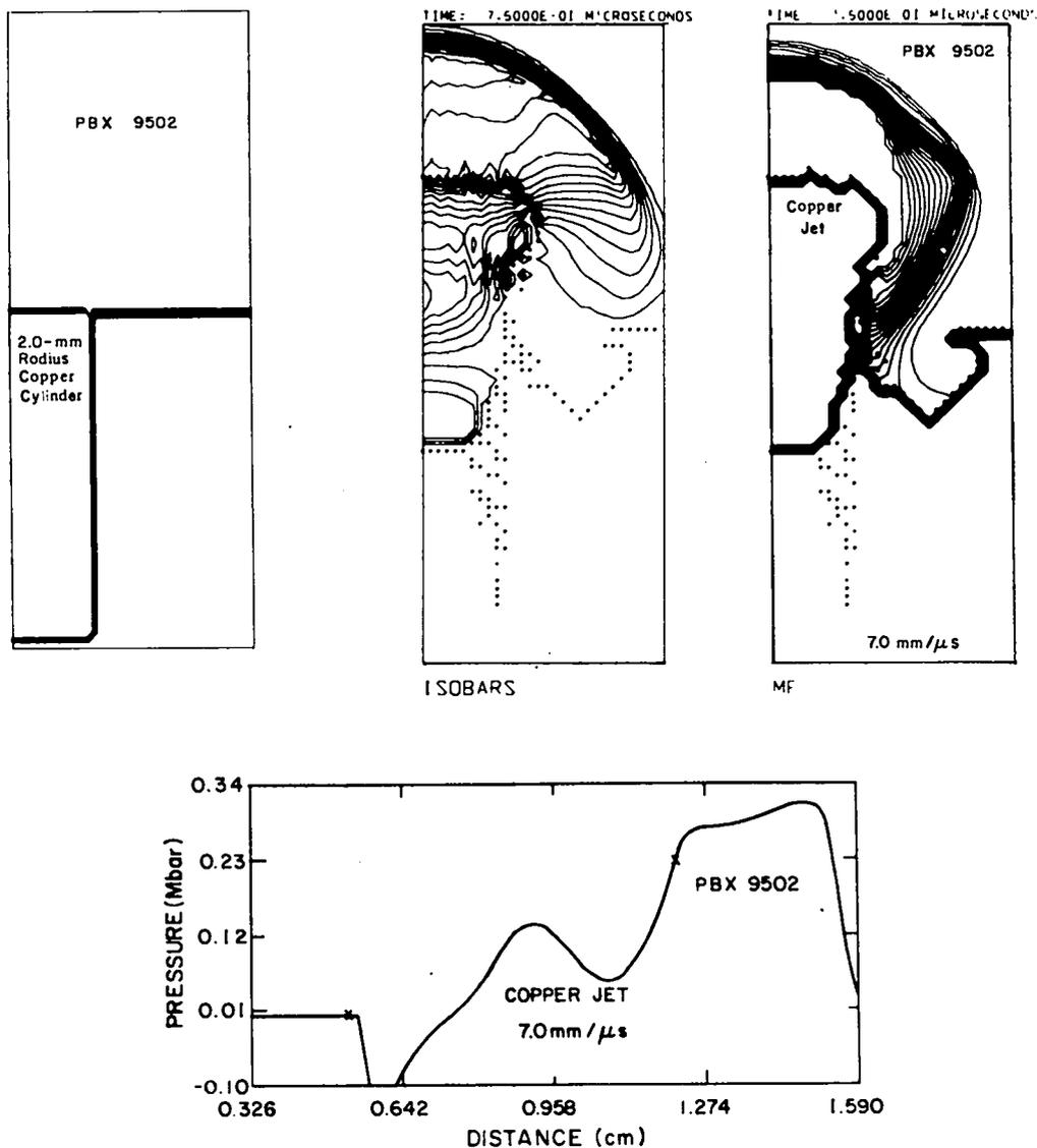
Fig. 4. The initial profile and the pressure and mass fraction profiles for a 4-mm-diam copper jet of 7.0 mm/μs shocking PBX 9502 at 0.75 μs. The isobar contour interval is 20 kbar and the mass fraction contour is 0.05. The pressure profile along the axis is also shown.
