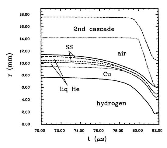
Fig. 9. Interface positions of 2nd cascade and central cryostatic sample container from RAVEN simulation of a possible isentropic compression experiment driven by COMP-B
