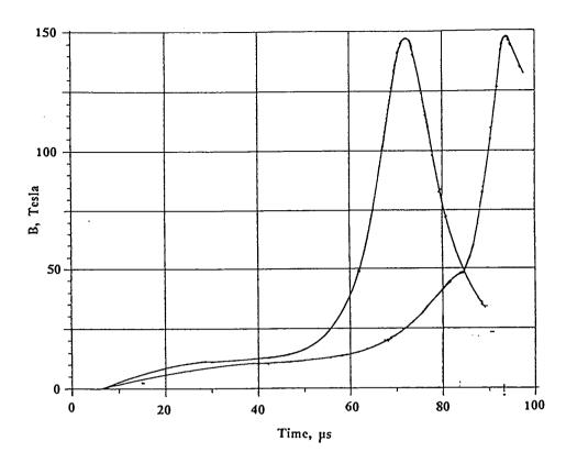
Fig. 10. Magnetic field vs. time plots from a single stage flus compressor (12.7 mm D load coil) and a two-stage compressor (28 mm D load coil).
