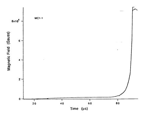
1) Faraday rotation measurements of the magnetic field for shot MC1-1. The solid line shows the flint glass results and the dashed line shows the results for a quartz sensor.
