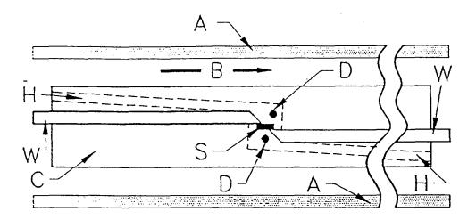
Fig. 11. Schematic of the diagnostics inside the MC-1 generator. A is the imploding liner, B is the magnetic field direction, C is the cryostat, D's are the temperature sensing diodes, H is the helium cooling channel, S is the sample, and W is the dielectric waveguide. The inductive and Faraday magnetic field probes are near D.
