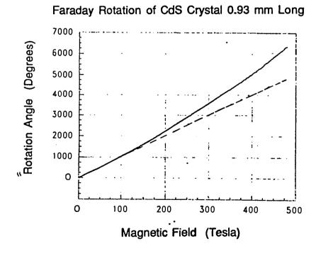
6) Faraday rotation in CdS (curve) v. magnetic field for shot MC1-5. The dashed straight line is drawn to help show the deviation from linearity at high fields.
