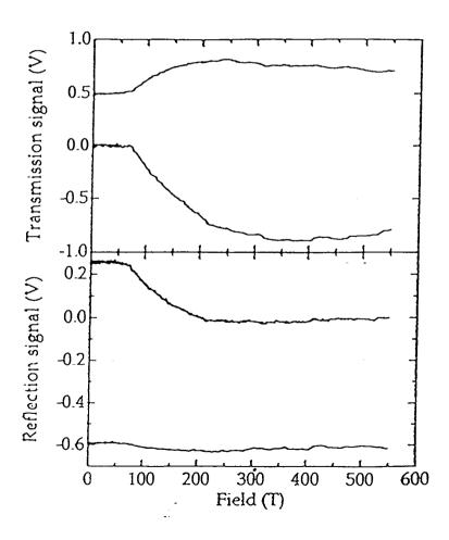
Fig. 12. Measured microwave transmission and reflection signals from the 4 K experiment plotted against magnetic field.
