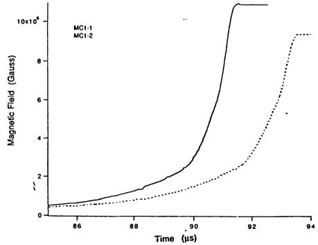
4) Faraday rotation measurements of the magnetic field from shot MC1-2. For comparison with the Comp-B-loaded shot, MC1-1, the dashed line shows the data of Fig. 1 delayed by 2.89  $\mu s$  so that the times after detonation are the same. The higher explosive energy of 9501 is demonstrated by the faster implosion and higher final field in shot MC1-2.
