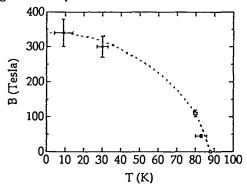
Figure 4. Measured values of B (points), the upper critical magnetic field in the superconductor YBCO, as a function of temperature. The one open point is from earlier work.
