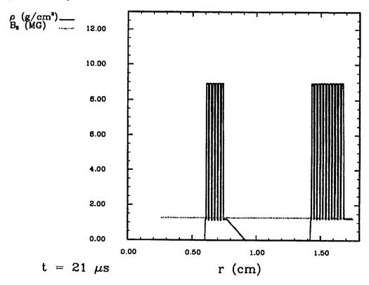
Fig. 4. Density and magnetic field profiles through the 2nd and 3rd cascades from RAVEN simulations of the MC-1 driven by COMP-B at 21 µs after HE detonation.
