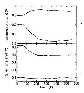
Figure 2. Measured microwave transmission and reflection signals from the 4 K experiment.
