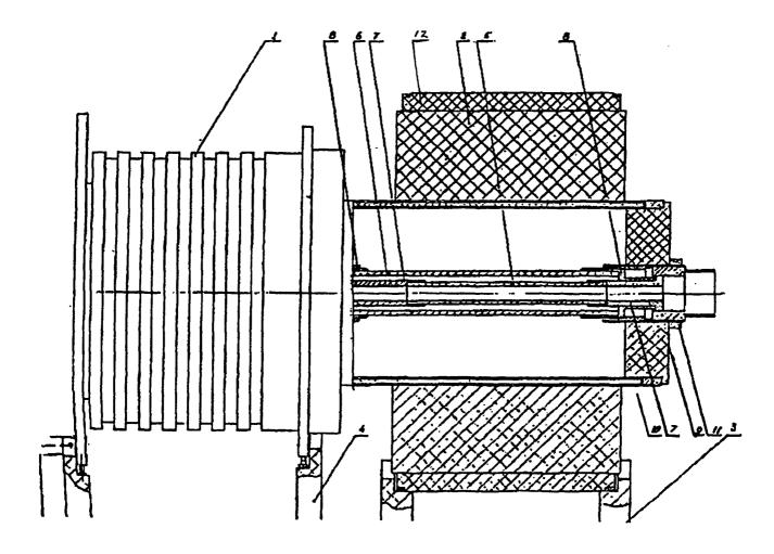
Fig. 1. Russian 3-cascade MC-1 FCG. Labels are identified as follows: 1 - insulated current feed for solenoid; 2 - explosive charge; 3, 4 - support stands; 5 - 3rd cascade; 6 - 2nd cascade; 7, 8, 9-insulating foam assembly cradles for cascades; 10 - solenoid; 11 - assembly nut; 12 - initiator
