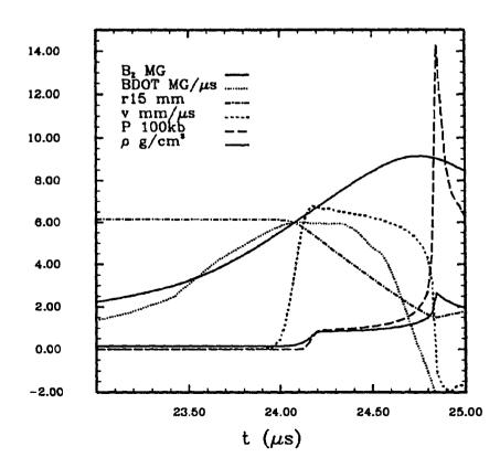
Fig. 8. Time history of the Lagrangian zone intially nearest 6-mm radius in the foam cryostat.
