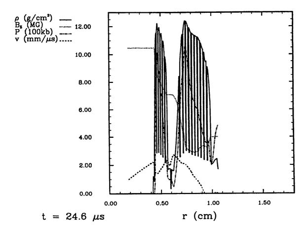
Fig. 6. Profiles through the 2nd and 3rd cascades from RAVEN simulations of the MC-1 driven by COMP-B at 24.6 µs after HE detonation.
