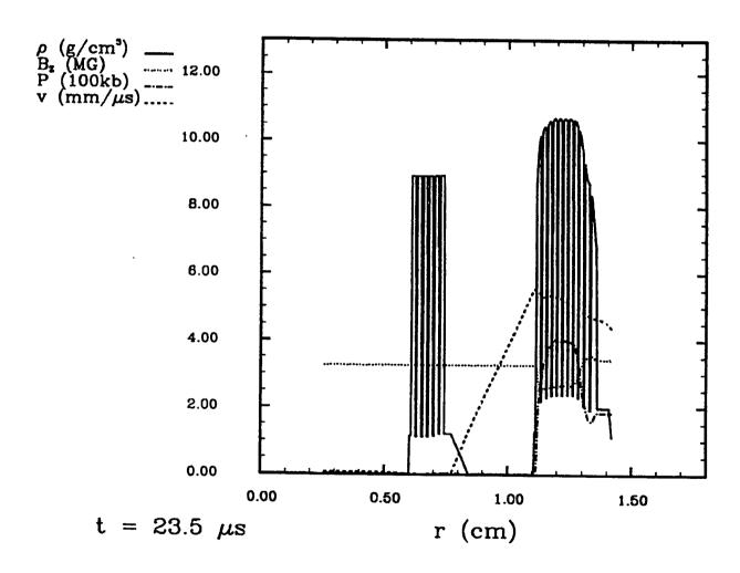
Fig. 5. Profiles through the 2nd and 3rd cascades from RAVEN simulations of the MC-1 driven by COMP-B at 23.5  $\mu s$  after HE detonation.
