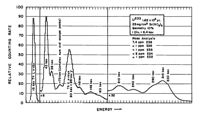
Figure 83. Gamma-ray spectrum of  $U^{233}$  obtained with a 4-inch diameter x 4-inch thick cylindrical NaI(T1) crystal. After C. E. Crouthamel, C. Gatrousis, S. J. Gaslovich, reference 649.
