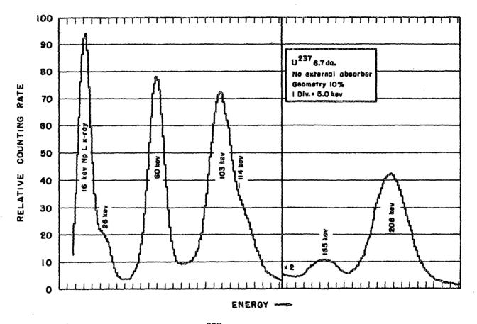
Figure 81. Gamma-ray spectrum of  $U^{237}$  obtained with a 4-inch diameter x 4-inch thick cylindrical NaI(T1) crystal. After C. E. Crouthamel, C. Gatrousis, S. J. Goslovich, reference 649.
