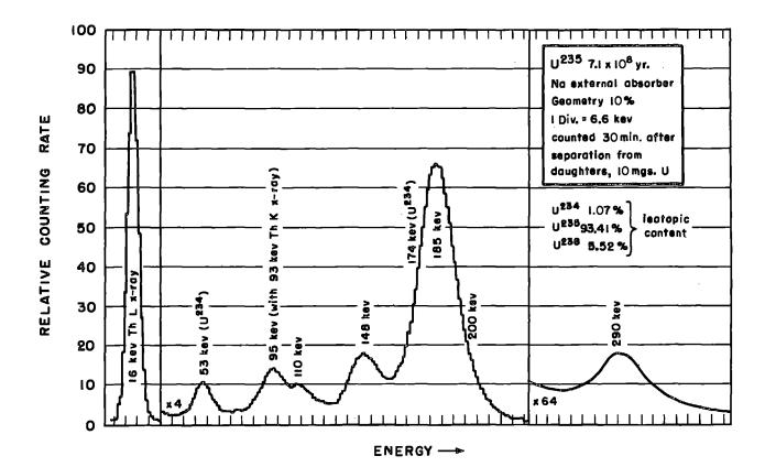
Figure 82. Gamma-ray spectrum of  $U^{235}$  obtained with a 4-inch diameter x 4-inch thick cylindrical NaI(T1) crystal. After C. E. Crouthamel, C. Gatrousis, S. J. Goslovich, reference 649.
