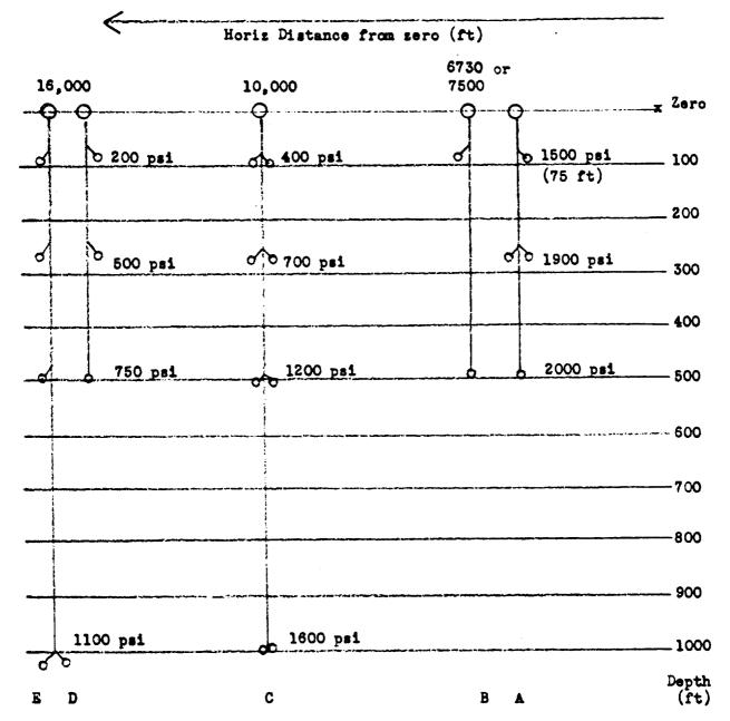
Instrument Line  $^{m}A^{m}$  is a 4-channel NOL system;  $^{m}B^{m}$ , a Hastings system;  $^{m}C^{m}$  is an 8-channel Wiancko system.
