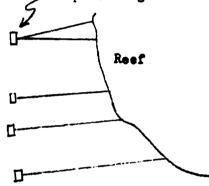
It is thought that a  $1-1/2^n$  chain should be sufficient to go from the moorings to the water. Then a  $1/2^n$  wire cable with breaking strength of 28,000 lbs will be adequate from the cable to the buoys. A deep sea moor will be put down to a 2800 lb anchor with a  $1-1/2^n$  chain leader. The instrument cans will be fastened to this system.
