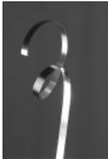
Los Alamos researchers achieved a breakthrough in superconductor technology with a piece of thin metal tape coated with a high-temperature superconducting material. The tape carries high current with no resistance at liquid nitrogen temperatures — even in high magnetic fields — and is flexible enough to be wrapped into a tight coil. The tape's flexibility and high current-carrying capacity give it a wide range of potential applications, including
