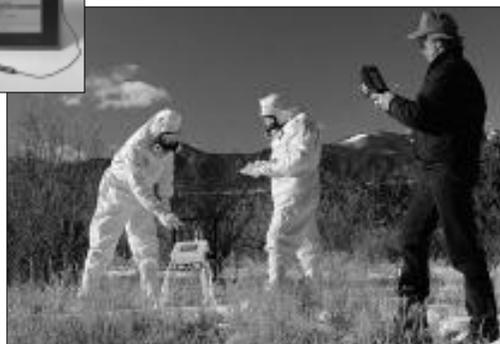
The system integrates off-the-shelf Global Positioning System, or GPS, electronics with a portable computer that includes notebook, pen, laptop, or palmtop and a software package developed by the inventors. Plume-in-
