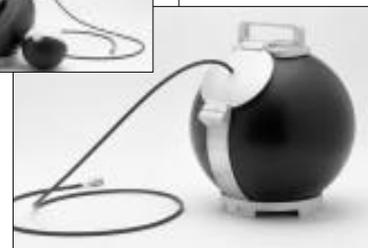
WENDI measures the amount of neutron radiation received by human beings with an accuracy and sensitivity unequaled by other neutron dose meters.
