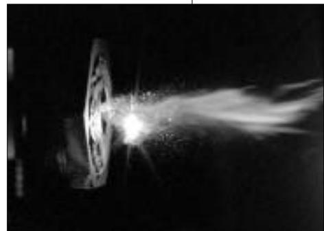
Specialized laser-light pulses are focused within a cloud of fuel to produce a laser-induced plasma, known as a "laser-spark," that ignites the fuel. The ability to reliably ignite fuel within the optimal zone of the engine's combustion chamber, in a manner unobtrusive to engine flow dynamics, will enhance the performance of existing turbojet engines as
