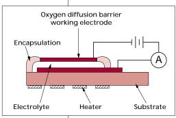
This technology involves the improvement of oxygen sensors that feed information back to the car's computer, thus allowing adjustments so that the fuel can burn more efficiently. Measuring the amount of oxygen coming out of the exhaust process and using that information to improve the way fuel burns avoids unburned hydrocarbons and greatly reduces air pollution.
